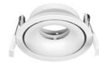
ENZO - 7201401 Sandy White Aluminium LED GU10 1x10 Watt IP20 220-240 Volt Bulb Excluded D: 10.5 H: 3.3 cm Cut Out: 10 cm
