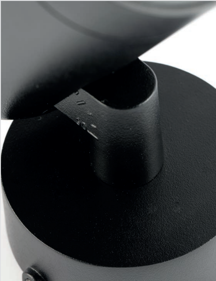
Goniometer built-into the luminaire arm for more precise aiming of the floodlight at the desired angle.
