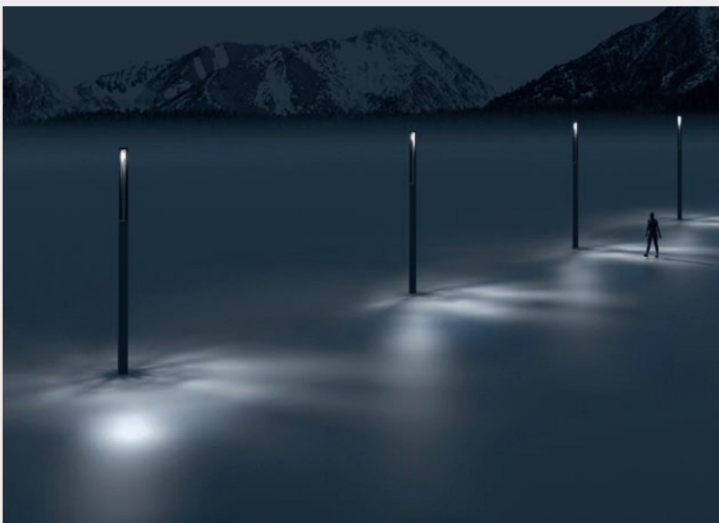
Simulation Screen 751312 38W 3000K Optics 360° Luminares interdistance 10mt.
